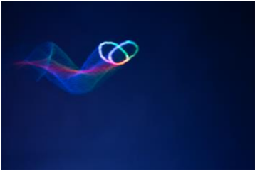
Figure 5: Acoustic levitation system [10] displays an abstract floating butterfly. A levitating particle is illuminated using RGB LEDs to control the color of the scattered light. Persistence of vision causes the glowing dot to appear as a continuous 3D image. Further, parametric audio and mid-air haptics are multiplexed in time and space to create a multimodal volumetric display. Picture credit: Eimontas Jankauskis University of Sussex.
